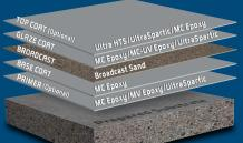
TOP CORT Ultra HTS/UltraSpartic GLAZE COAT MC-UV Epoxy/UltraSpartic 2""BROADCAST 2<sup>nd</sup> BRSE CORT Quartz Granules MC Epoxy/MC-UV Epoxy 1"<sup>®</sup>BROADCAST 1<sup>st</sup> BRSE CORT Quartz Granules PRIMER (Optio MC Epoxy/MV Epoxy/UltraSpartic
