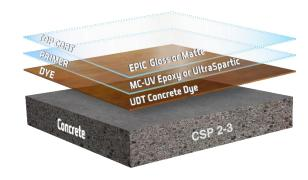
EPIC Grind, Dye, and Seal
