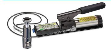
Measures the adhesion of a coating to a surface by pulling an aluminum "dolly" that has been glued to the surface until failure, ideally of the substrate. Very effective for cementitious flooring and terrazzo. Measure in PSI, dollies are typically 10, 20 or 50 mm. UDT standard is a 20mm dolly.
