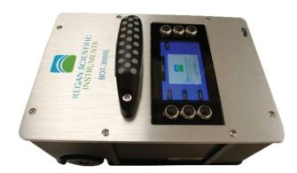
Test method for measuring dynamic coefficient of friction (DCOF) on hard surface materials. Automated method to ensure applicators are meeting recommended slip resistance parameters of the American National Standards Institute (ANSI). Slides a small "shoe" across a surface that has a surfactant present, test is repeated from several angles to ensure accurate readings.
